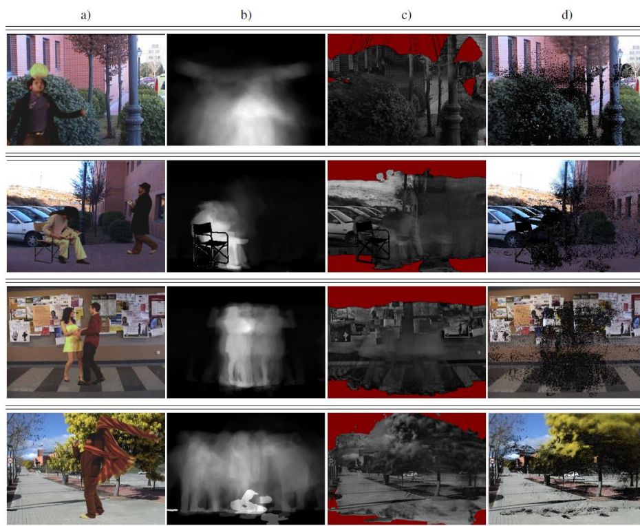
Figure 9. Videos extracted from [40]. a) Example frame, b) Foreground evolution, c) Average difference between foreground and background (red areas are never foreground), d) Prone to camouflage pixels (in black).
